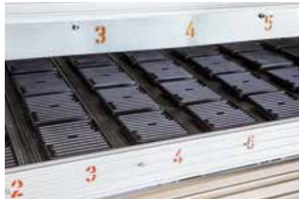
Heating with efficient ceramic elements (HTS)
