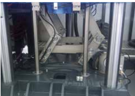
Lower drive cutting station with tension bars
