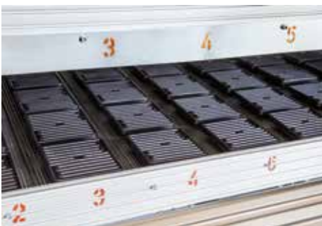
Heating with efficient ceramic elements (HTS)
